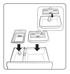
**3.** Remove the inserts from the 3 compartments. Rinse the inserts and the drawer with warm water to remove traces of accumulated laundry products.
