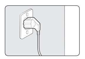
Plug the power cord into a 3-prong, well grounded 230 volt 60 Hz approved electrical outlet protected by a fuse or comparable circuit breaker.
