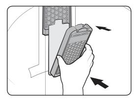
**3.** When cleaning is complete, close the cover and reinsert the filter case to the original position. You will hear a clicking sound when the filter case fits in.
