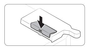
**4.** Insert the upper area of the adapter cover first, and then close to lock as shown.
