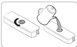
2. Fill the water tank with potable water up to 2.8 liters. You can remove either the top cap or the cover and pour water.
