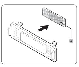
While holding the top and bottom sides of the filter case, unlock the filter case to reveal the **deodorizer filter (A)**. Replace the filter, and then reinsert the case.
