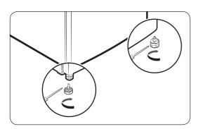
Level the refrigerator by manually adjusting the levelling feet. Turn the levelling feet clockwise to lower the position, or turn counter clockwise to raise.
