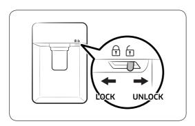
**4.** Put a water glass under the water outlet of the dispenser, and gently push the dispenser lever to dispense water. Make sure the water dispenser is unlocked.
