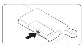
**1.** Press to unlock the arrow area of the adapter cover.
