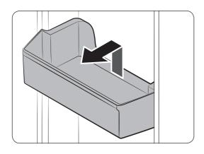
Slightly lift up and pull out the door bin.
